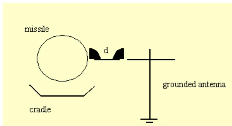
Assume that the missile and the cradle formed a parallel plate capacitor with an effective area of 4.0 square feet and a plate separation of 6.0 inches. The average surface charge density  $\sigma$  is  $1.0 \times 10^{-9}$  Coulombs per square meter. The breakdown electric field strength of cold dry air is  $3.0 \times 10^6$  V/m.
