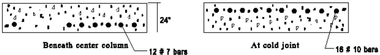
4. If a "cold joint" actually existed at the point shown in Figure 1, assume the footing will behave as if a hinge were there. Write a brief qualitative description of the likely result of such a hinge if an earthquake produces the lateral loads shown in Figure 1.
